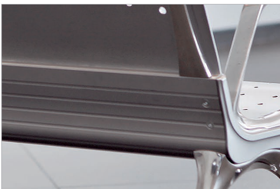
Extruded aluminium central beam 135 height and 202 mm depth 5 mm thickness
